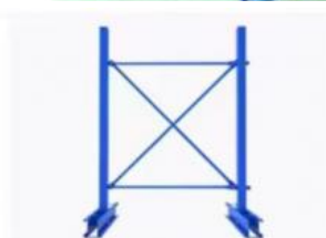
Step 3: Install connecting rod
